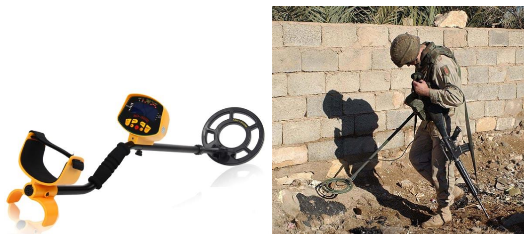
Fig. 6. Modern handheld computerized induction balance metal detectors. The LCD screen is a standard among the high-end metal detectors nowadays.
