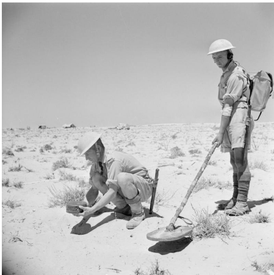
Fig. 5. Mine detector Mark I used by sappers of the Royal Engineers corps, North Africa, 28 August 1942.
