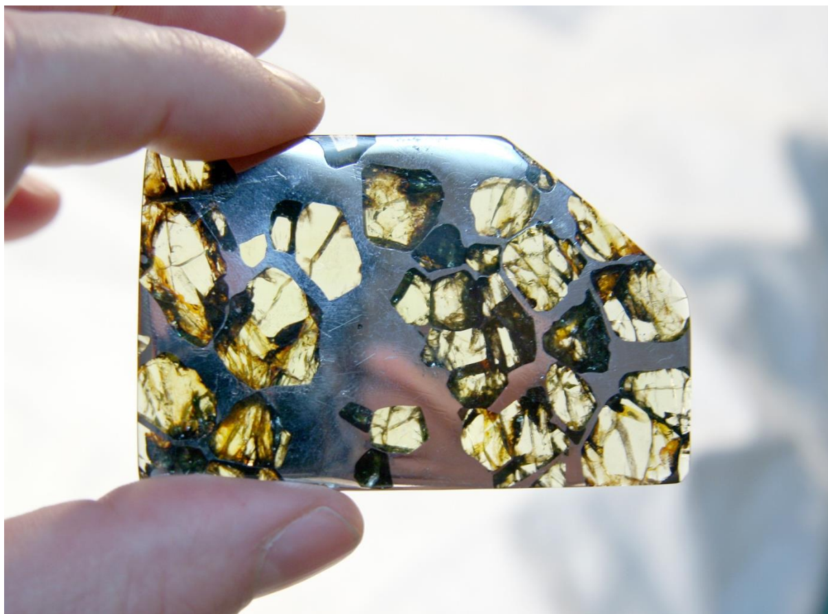
Fig. 3. A slice of the Esquel meteorite (pallasite). This type of meteorite is from the core-mantle boundary of an ancient planetoid that was smacked apart billions of years ago. The metal is iron/nickel core material and the crystals are peridot from the mantle area. At the interface, they mix together as you can see. Author Doug Bowman.
