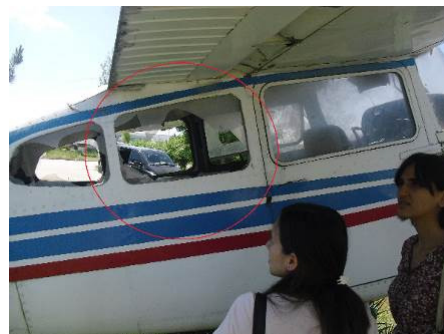
Figure 6. Broken windows of the plane causes safety barrier to the material
