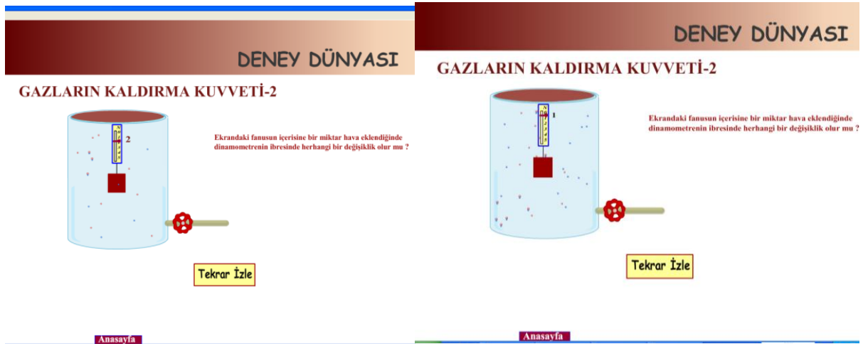
Figure D.4. Animation print-screen views describing the relationship between gas density and buoyancy force exerted on the object
